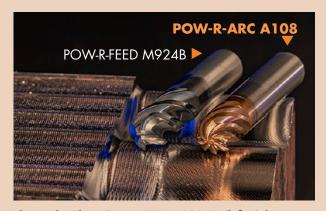
The tools: The POW-R-FEED M924B (left, 3/4 in. dia., 4-flute ball end, 1 in. LOC) v. the POW-R-ARC A108 (right, 3/4 in. dia., 8-flute ball end, 1 in. LOC) Material: A2 at 60 HRc. Using the same stepover value, the new POW-R-ARC 8-flute tool provides a superior 3D contour cut 5x faster, with barely visible ridges (far right) and very little finish work.
